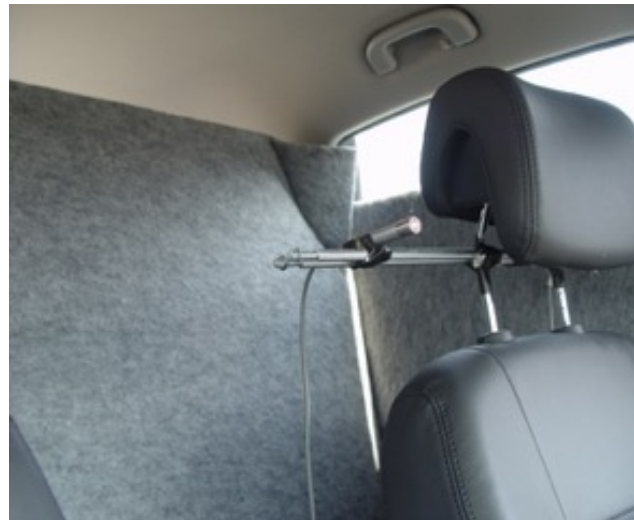
Vehicle rear prepared with absorber felt to reduce reactive intensity
