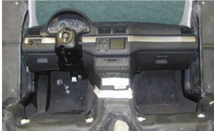
Complete vehicle front-end in STL test window (view from receiving room)
