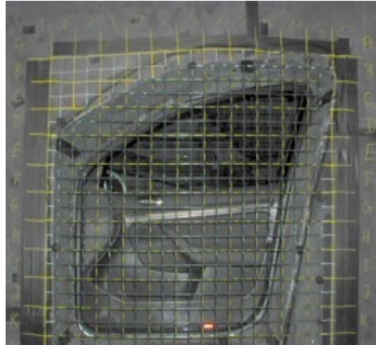
Vehicle door in STL test window (view from receiving room)
