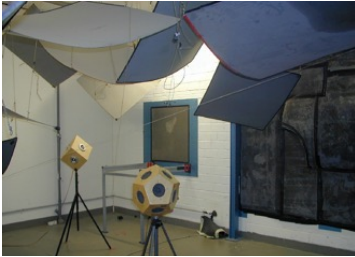
Reverberation room with diffusers, small & large STL test window
