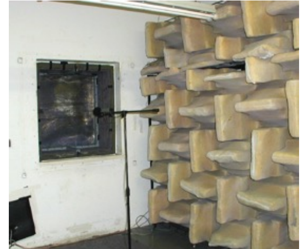
Small STL test window for material & component tests
